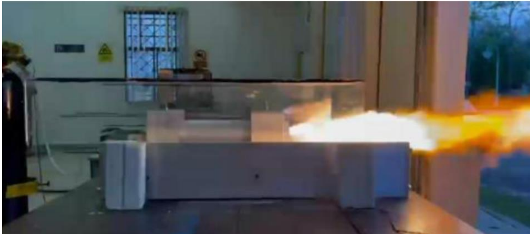
Figure 9: Single port with oxidizer pressure of 100 kPa
