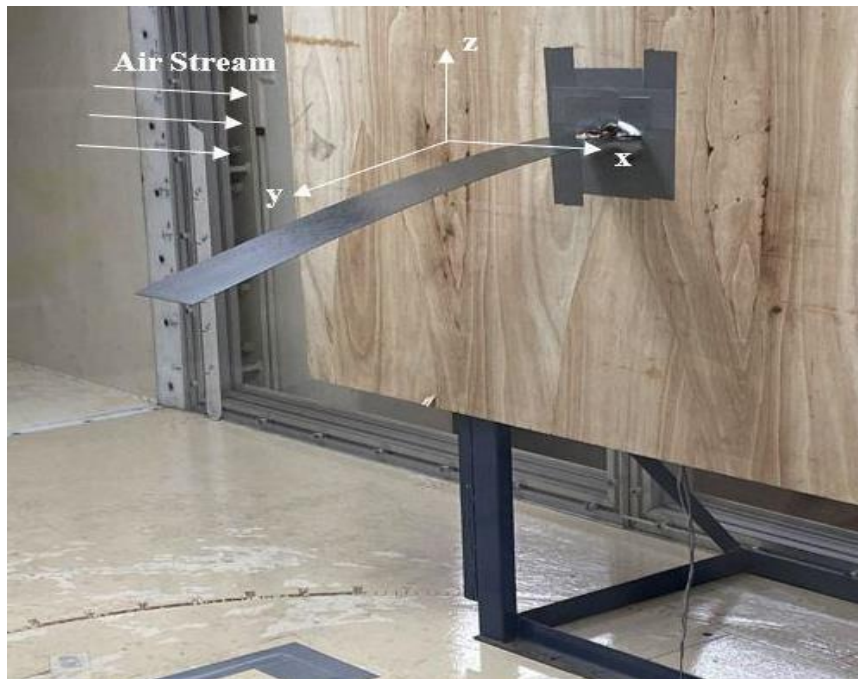
Figure 3: Experimental set-up in the test section of the wind tunnel
