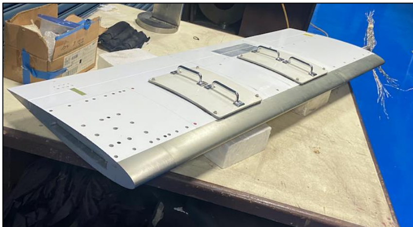
Figure 1: NACA-0012 model used for this flow control study
