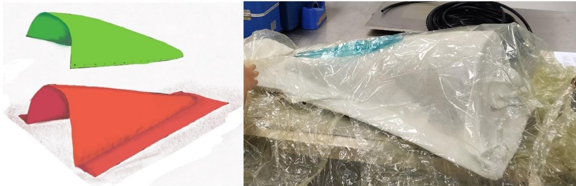
Figure 6: Positioning of the repaired panel on top of the mold and the vacuum bagging encapsulation during curing
