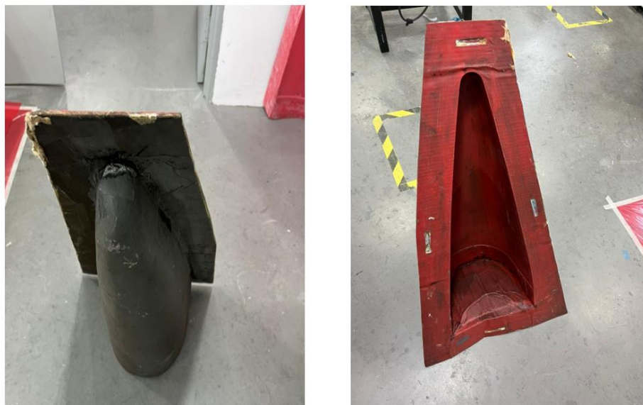
Figure 5: Fabrication of in-house male mold to support the part during curing
