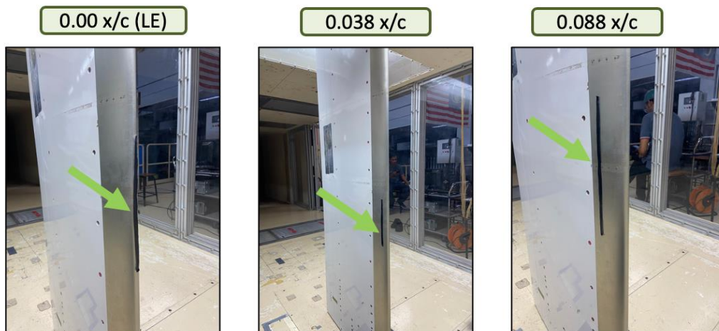
Figure 3: Considered strip locations for the parametric study
