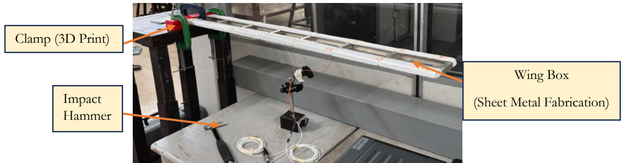
Figure 2: Experimental modal analysis (EMA) setup
