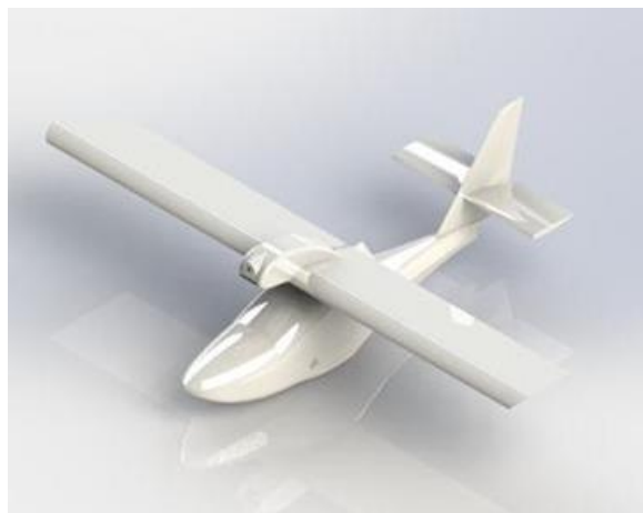
Figure 2: Constructed CAD model of the Borey seaplane
