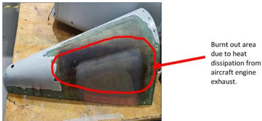
Figure 3: Extent of damage that is observed on the IFFF component
